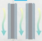
The fan operation after shut down helps dry water droplets to keep the coils dry
